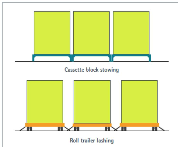
Figure 4. Stowing of cassettes and roll trailers
